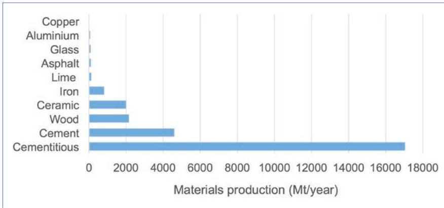
**Figure 2.** Estimated consumption of common materials 2002–2005. Data from [10,11]. Except from ceramics, asphalt and cementitious, all other materials are shared with other industries. Part of wood is used for fuel and furniture.
