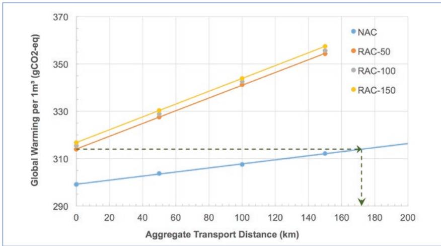
**Figure 18.** The effect of transportation distance on associated CO<sub>2</sub> emissions of concretes produced with recycled aggregates and natural aggregates. The substantial difference results from tested recycled aggregates requiring much higher cement content to reach the necessary design strength [47].
