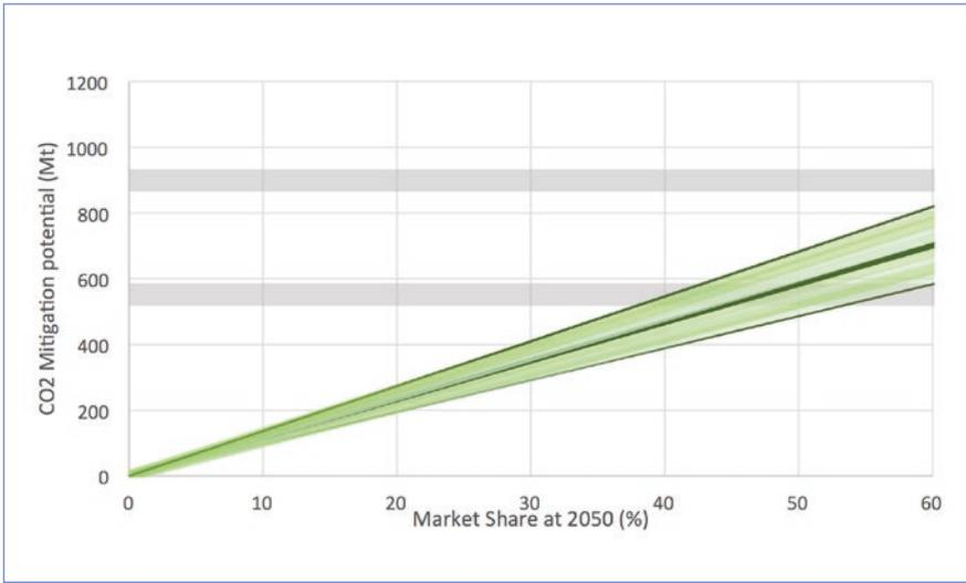
Figure 22. Mitigation potential of filler substitution, varying between 25–35% as a function of market share for the 2050 low demand scenario. High filler amount will require dispersant use. Horizontal lines represent (for reference) the mitigation targets from the 2DS scenario for CCS and in total.
