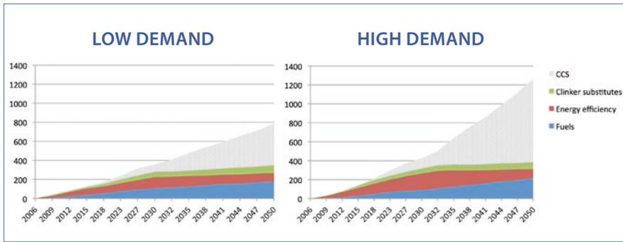
Figure 4. Cement sector CO<sub>2</sub> emissions reductions below base line 2006–2050, adapted from 1.8% [Tam, C and Van der Meer, R, IEA/CSI technology roadmap for the cement industry, 6th International VDZ Congress 2009, pp. 155–157]
