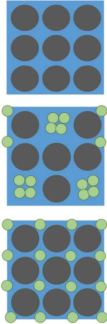
**Figure 15.** The effect of the combination of binder replacement by inert fillers. Without the presence of the dispersant admixture (centre), as is usual in today's cement industry, ultrafine filler agglomerates may increase the water demand. Dispersants destroy the agglomerates (right), and if the particle size distribution is adequately engineered, will reduce the amount of water needed to fill intergranular space and separate the particles.
