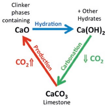
**Figure 9.** The Cement/Concrete carbon cycle, “chemical” CO<sub>2</sub> emitted during production from limestone breakdown is proportional to CO<sub>2</sub> reabsorption capacity during carbonation.
